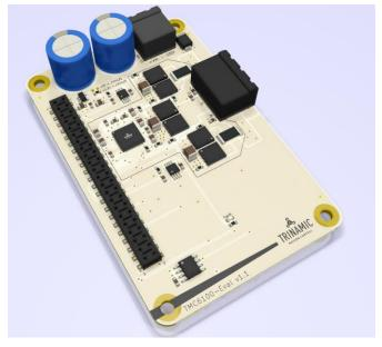
A CPU with internal BLDC or sine wave PWM unit drives the gate control lines based on encoder or hall sensor feedback. External current sensing is required, either using simple Op AMPs for foot point sensing, or series shunt amplifiers. Use of SPI is not required unless more sophisticated diagnostics is desired.
