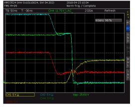
Figure 3.8 Ringing of output (green) and Gate voltages (yellow, blue) with DRVSTRENGTH=2
