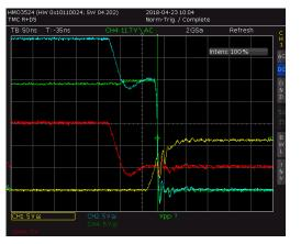
Figure 3.9 Ringing of output (green) and Gate voltages (yellow, blue) with DRVSTRENGTH=3
