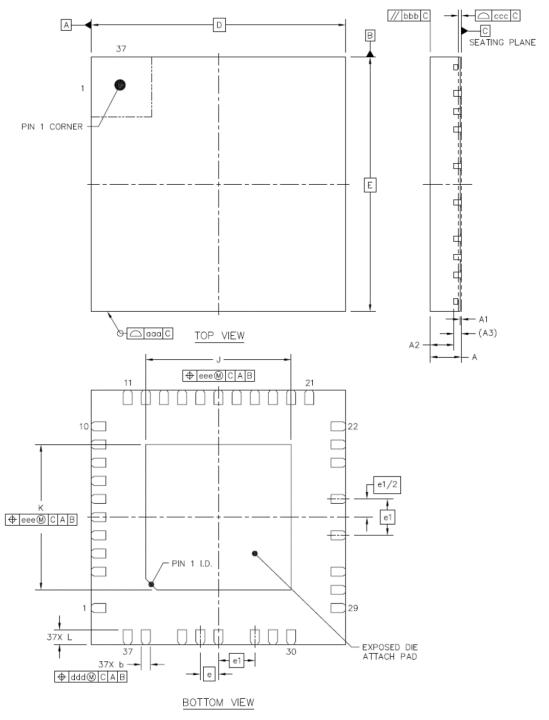
Figure 12.1 Dimensional drawings QFN7x7
