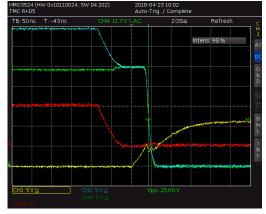
Figure 3.7 Ringing of output (green) and Gate voltages (yellow, blue) with DRVSTRENGTH=0
