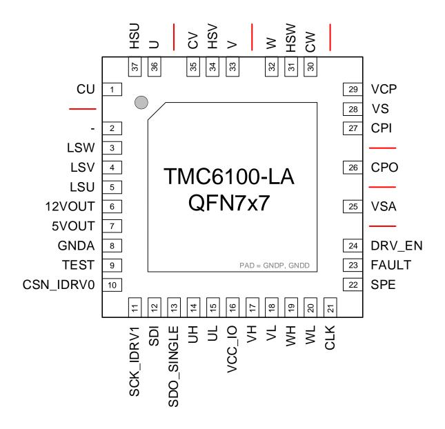
Figure 2.1 TMC6100-LA pinning QFN 37 special (7x7mm²)
