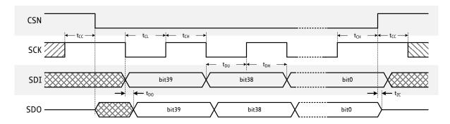
Figure 4.1 SPI timing
