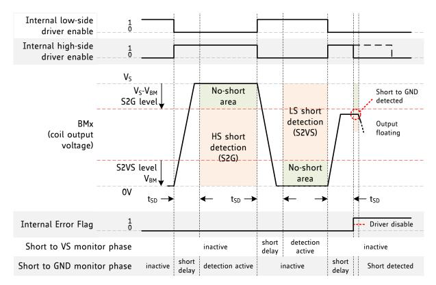
Figure 6.1 Short detection (U, V or W output)
