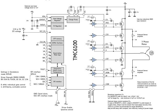
Figure 3.1 Standard application circuit
