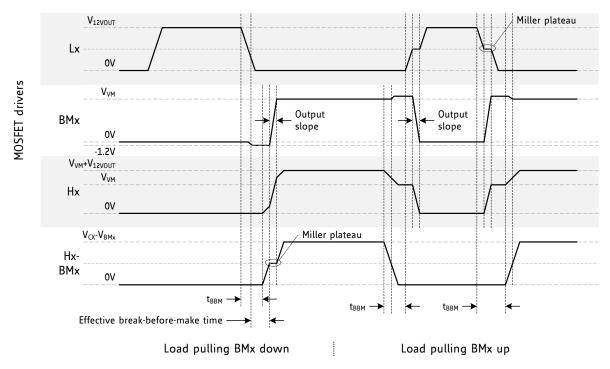
Figure 3.5 Slopes, Miller plateau and blank time (BMx=U V or W output)
