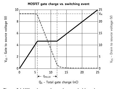
Figure 3.4 Miller charge determines switching slope
