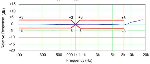
Typical Free Field Response Normalized to 1kHz Low Power Mode  $V_{DD}$ =1.8V,  $f_{CLK}$ =768kHz, Decimation Rate=64x
