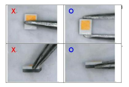
3. There are no restrictions on the form of the pick and place nozzle, except that mechanical stress on the surface of LED must be prevented. Lextar recommend that the material of nozzle is the rubber or the silicone, which the property is soft to prevent break the LED.
