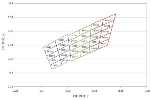
Tolerance of measurements of the Chromaticity Coordinate is  $\pm 0.005$ .
