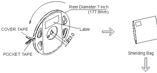
Maximum 5 bags in 1 inner box Inner box dimension = 290mm x 240mm x 70mm
