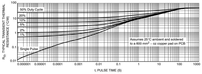
Figure 8. Typical Thermal Characteristics
