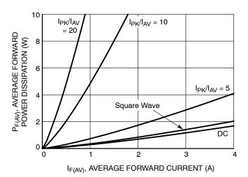
Figure 7. Forward Power Dissipation
