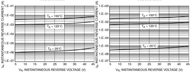
Figure 3. Typical Reverse Characteristics Figure 4. Maximum Reverse Characteristics
