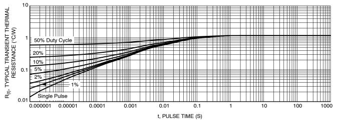
Figure 9. Typical Transient Thermal Response Characteristics, Junction-to-Case
