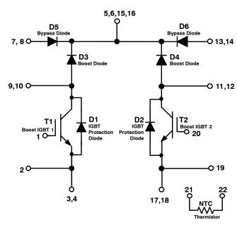
Figure 1. NXH80B120H2Q0SG Schematic Diagram
