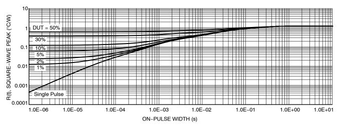
Figure 16. Diode Transient Thermal Impedance Boost Diode
