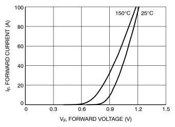
Figure 19. Diode Forward Characteristic
