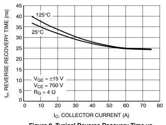
Figure 9. Typical Reverse Recovery Time vs. IC
