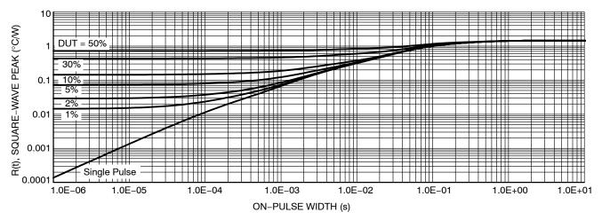
Figure 20. Diode Transient Thermal Impedance Bypass Diode / IGBT Protection Diode
