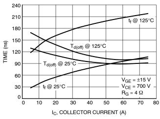
Figure 7. Typical Switching Times vs. IC
