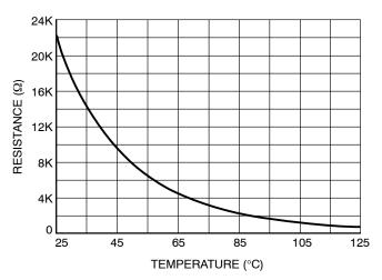
Figure 21. Thermistor Characteristic
