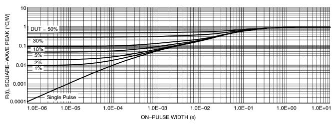
Figure 15. IGBT Transient Thermal Impedance
