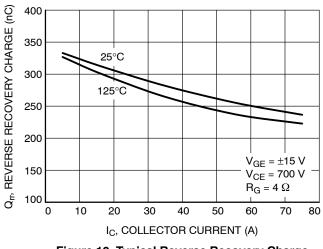
Figure 10. Typical Reverse Recovery Charge vs. IC
