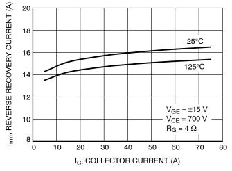
Figure 11. Typical Reverse Recovery Peak Current vs. IC
