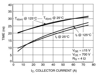
Figure 8. Typical Switching Times vs. IC
