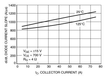
Figure 12. Typical Diode Current Slope vs. IC
