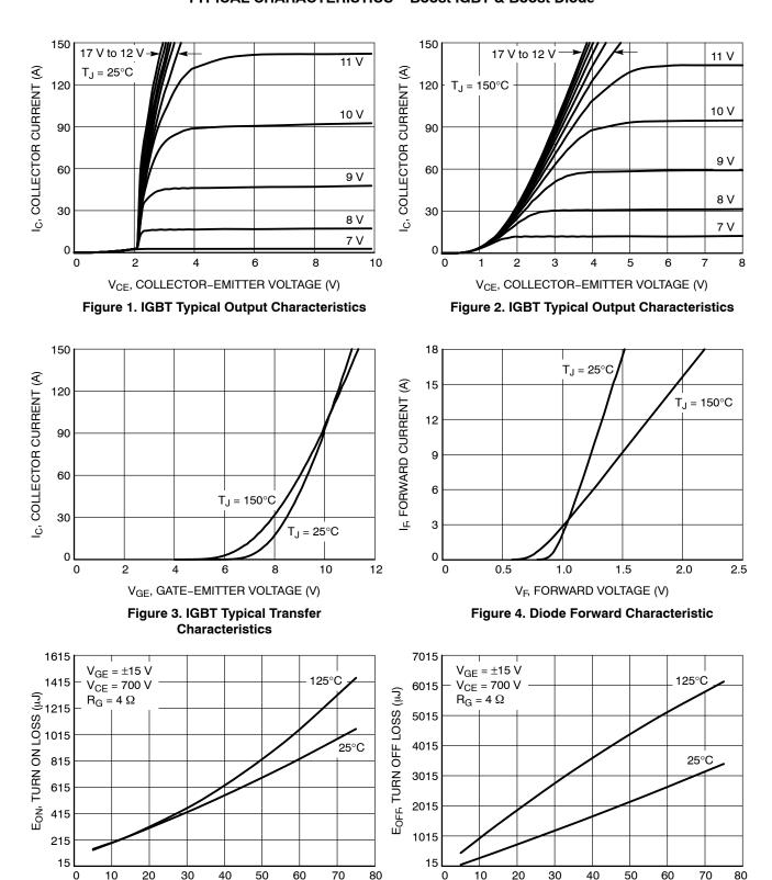
$I_{C}, \mbox{ COLLECTOR CURRENT (A)} \label{eq:collection}$  Figure 5. Typical Turn On Loss vs. IC
