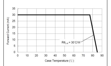
Solder Temperature (Slug) vs. Maximum Forward Current
