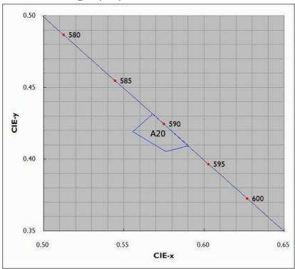
Tolerance of measurements of the Chromaticity Coordinate is  $\pm 0.005$ .
