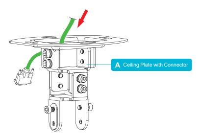
Feed the projector cable(s) through the top of the Ceiling Plate.
