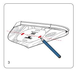
Using the marking template provided, mark two holes for drilling on the centerline of the stud.
