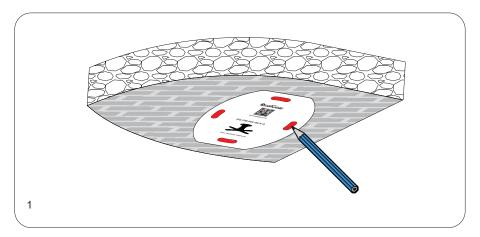
Hold the marking template provided against the ceiling where you want to install the projector, mark four holes for drilling.
