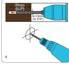
Using a power drill and 3/16" drill bit, drill pilot holes of 3/16" (4.5 mm) diameter and at least 2.5" (65 mm) depth.
