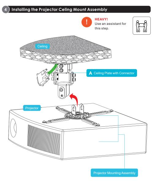
Align the Projector Mount Assembly to the Ceiling Plate with Connector, then using the Alley Key (M-P), attach them together with the provided Screws (M-M), Washers (M-N), and Plastic Washers (M-O).
