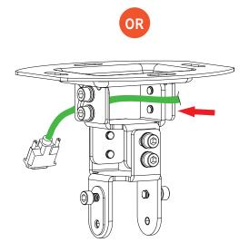
Feed the projector cable(s) through the side of the Ceiling Plate.
