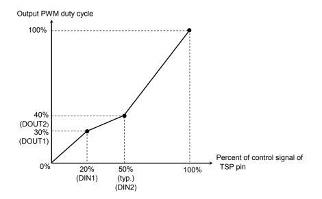
To set the above relation between the percent of control signal of TSP pin and the output PWM duty cycle, set the level of SEL\_ADJ pin and the voltage of ADJ0 pin, ADJ1 pin and ADJ2 pin shown below.
