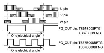
$\cdot$  Timing Chart of the Motor Driving signals in rotation of forward direction
