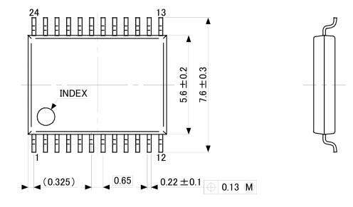
Detail figure of pin tip shape
