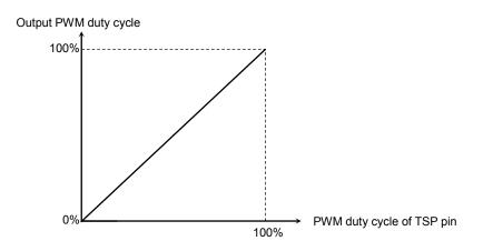
Note: The relation when ADJ1 pin and ADJ2 pin are connect to ground is shown above. For details of ADJ1 pin and ADJ2 pin, refer to 5.3
