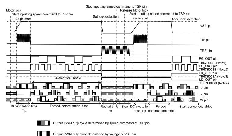
4) Timing chart of stopping speed command of TSP pin during lock detection
