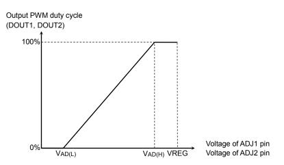
Note: Voltage setting of ADJ1 pin and ADJ2 pin should be set as follows; voltage of ADJ1 pin ≤ voltage of ADJ2 pin. If it is set as follows; voltage of ADJ1 pin > voltage of ADJ2 pin, this function may not operate correctly.
