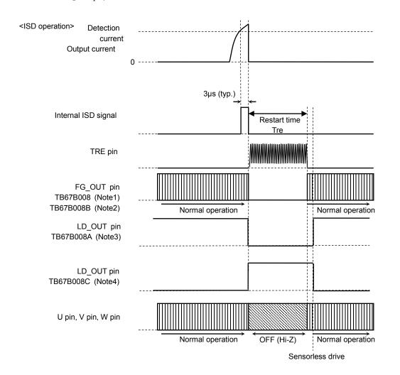
Note: When the ISD circuit is activated, the output current is more than the absolute maximum current rating. This circuit is provided as an auxiliary only and does not necessarily provide the IC with a perfect protection from damages due to over current caused by power fault, ground fault, load-short and the like.
