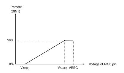
3) When the percent value of the control signal is equal or less than the duty cycle (DIN1) specified by a voltage of ADJ0 pin, the relation between the percent value of the control signal and output PWM duty cycle according to the state of SEL\_ADJ pin is shown in the below table.
