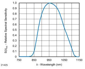
Fig. 3 - Relative Spectral Sensitivity vs. Wavelength
