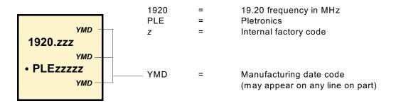
The actual part number is TCD4025-19.20M where the model number "025" is the specification number the part is made to. This is not included in the part marking. This is included on the label on the Tape and Reel.
