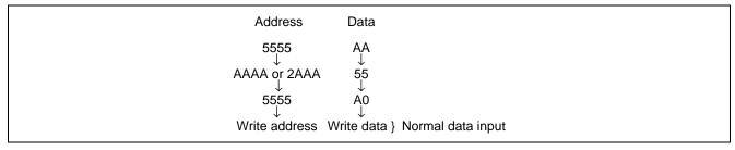
The SDP mode is disabled by inputting the following 6 bytes code. Note that, if data is input in the SDP disable cycle, data can not be written.
