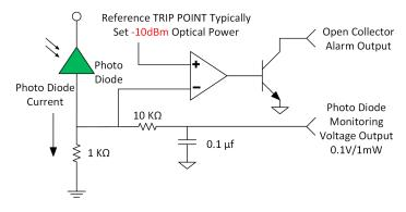
All alarms are Open Collector topology, with Active Low for Normal operations and during Alarm condition the open collector will Pull to High logic levels. Reverse polarity alarm is also available upon request, such as under normal conditions the Open collector will be High and vice versa under fault conditions.
