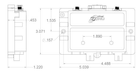
RF Connector = SMA Female Optical Connector = SC/APC or FC/APC DATA + ALARM = DB9
