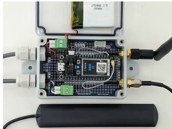
Pic. 18. LiPol battery applied to a transparent lid (inside view)
