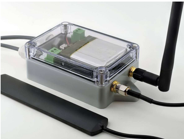
Pic. 17. LiPol battery applied to a transparent lid (assembled view)
