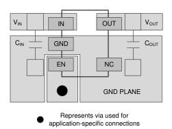
Figure 38. Layout Example for the DBV Package
