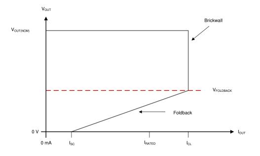
Figure 28. Foldback Current Limit
