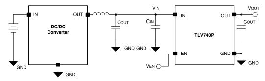
Figure 34. Operation From a DC/DC Converter
