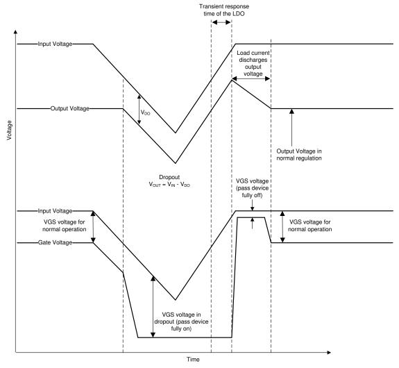
Figure 31. Line Transients From Dropout
