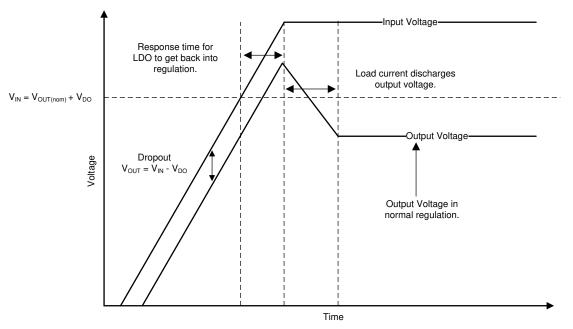
Figure 30. Start-Up Into Dropout
