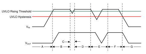
Figure 29. Typical UVLO Operation
