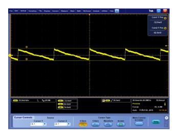
**Figure 4-2** Vin=230Vac, V=50mV/div, H=20ms/div Vout ripple=74mVp-p, Pout=0W
