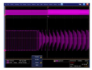
**Figure 9-2** ACF to DCM in 100Vac, V=50V/div, H=40us/div
