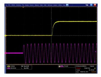
**Figure 5-2** Vin=230Vac, V-5V/div, H=50ms/div
