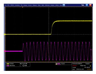
Figure 5-4 Vin=230Vac, V-5V/div, H=50ms/div
