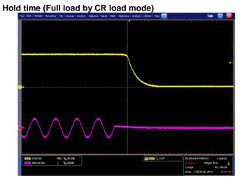
Figure 6-1 Vin=100Vac, V=5V/div, H-20ms/div
