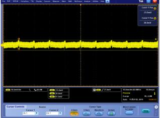
Figure 4-3 Vin=100Vac, V=50mV/div, H=10ms/div Vout ripple=61mVp-p, Pout=102W
