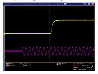
Figure 5-3 Vin=100Vac, V=5V/div, H=50ms/div
