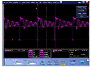
**Figure 8-3** Max voltage of Vsw in DCM operation, V=100V/div, H=10us/div, Vsw=518V/div, f=47.8 kHz
