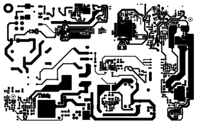
**Figure 14-4** Top view of layer 4 (Bottom layer)
