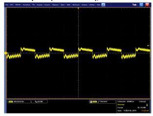
Figure 7-1 Vin=100Vac, V=200mV/div, H=5ms/div
