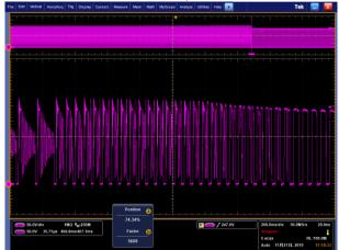
**Figure 9-1** DCM to ACF in 100Vac, V=50V/div, H=35us/div
