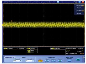
**Figure 4-4** Vin=230Vac, V=50mV, H=10ms/div Vout ripple=68mVp-p, Pout=102W
