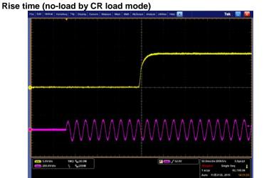
Figure 5-1 Vin=100Vac, V=5V/div, H=50ms/div
