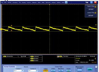
**Figure 4-1** Vin=100Vac, V=50mV/div, H=20ms/div Vout ripple=50mVp-p, Pout=0W
