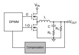
Figure 15. Control Loop Block Diagram
