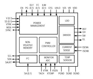
Figure 1. Block Diagram
