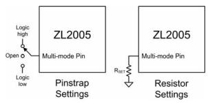
Figure 8. Pin-strap and Resistor Setting Examples
