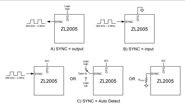
Figure 12. SYNC Pin Configurations
