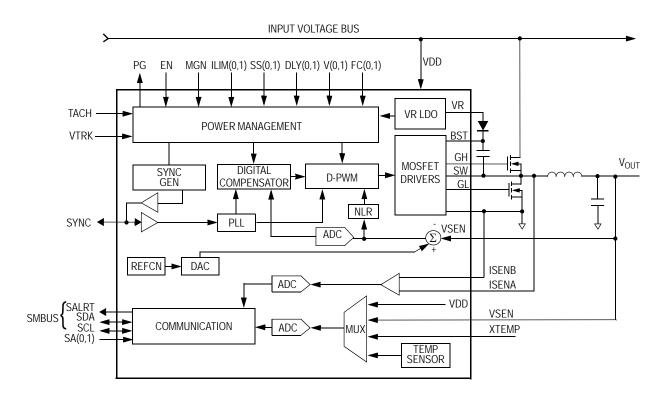
Figure 5. ZL2005 Detailed Block Diagram
