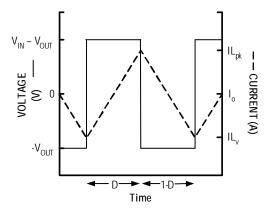
Figure 7. Inductor Waveform
