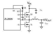
Figure 6. Synchronous Buck Converter
