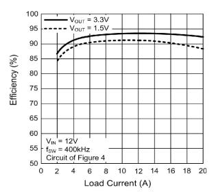
Figure 2. Efficiency vs. Load Current
