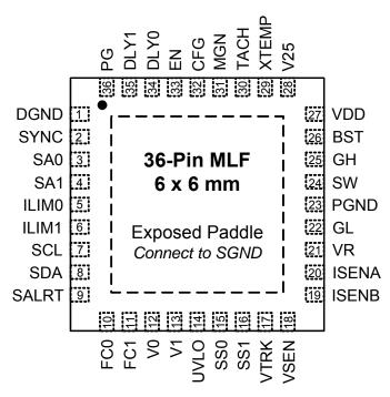
Figure 3. Pin Assignments (top view)
