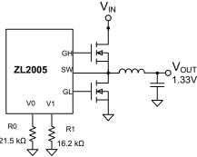
Figure 10. Output Voltage Resistor Setting Example
