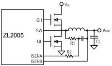
Figure 13. DCR Current Sensing
