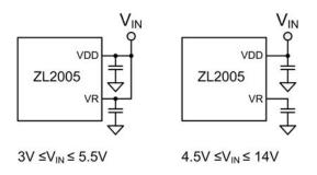
Figure 9. Input Supply Connections
