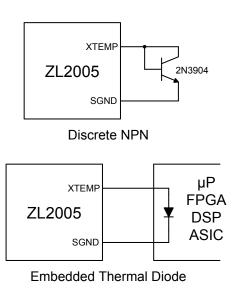
Figure 18. External Temperature Monitoring
