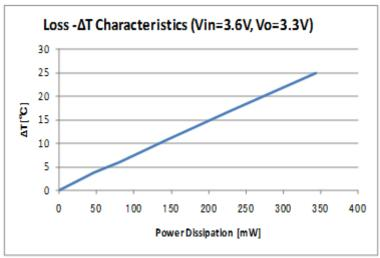
The output current of the device may need to be de-rated if it is operated in high ambient temperature or in an application that requires continuous power delivery. The amount of current de-rating is highly dependent on the environmental thermal conditions, e.g., PCB design, nearby components, or effective air flow. Care should especially be taken in applications where the device temperature exceeds 85°C.
