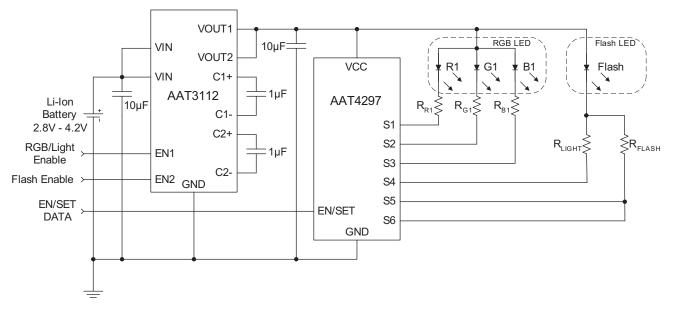
Figure 6: RGB LED Fashion Light With a Dual Mode Light/Strobe Flash LED Solution Using an AAT4297.
