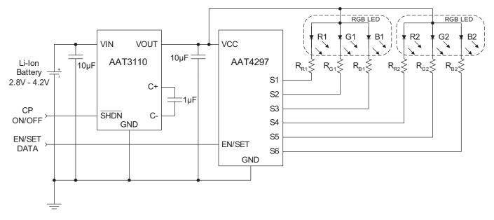
Figure 5: Dual RGB LED Fashion Light Solution Using an AAT4297.
