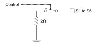
Figure 2: Simplified Equivalent Model.
