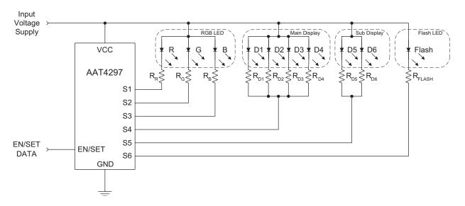
Figure 7: Total Lighting Control Solution Using an AAT4297. Includes RGB Fashion Light, Main Display and Sub-Display LCD Backlight, and Photo Flash LED.
