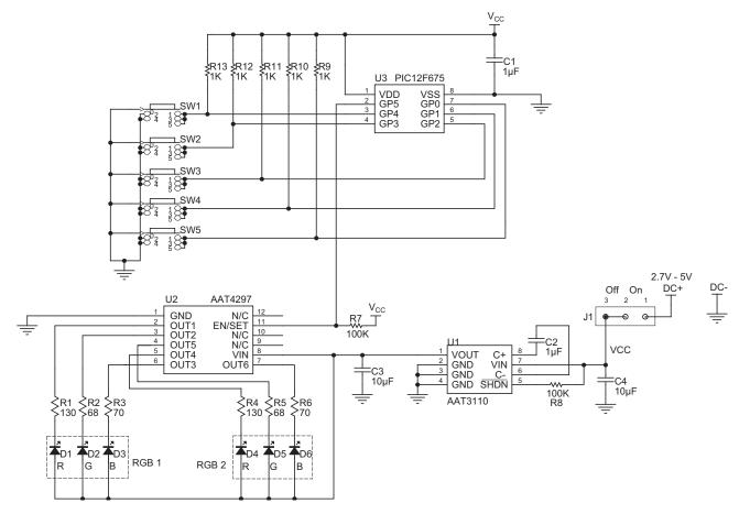
Figure 11: AAT4297 Evaluation Board Schematic.
