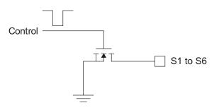
Figure 1: Switch Input Circuit.
