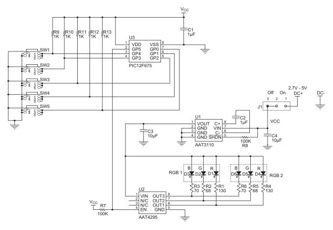
Figure 8: AAT4295 Evaluation Board Schematic.
