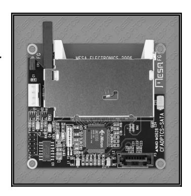
The CFADPT9 is a SATA to Compact Flash adapter on a small PCB. The form factor matches our CFADPTCS IDE to CF adapter.
