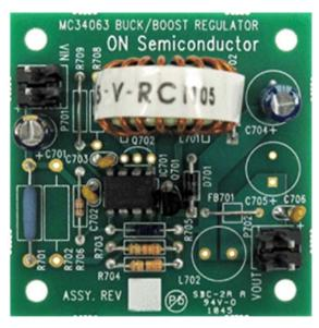
The MC34063 is a switching control circuit for use in DC to DC converters. With an on board switch capable of delivering 1.5 A, this versatile controller can be utilized in step up, step down, buck-boost, or voltage inverting topologies with a minimum number of components.
