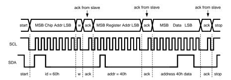
Figure 20. Write Cycle (w = write; SDA = '0'), id = device address = 60Hex for LP8755.
