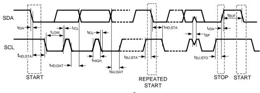
Figure 1. I<sup>2</sup>C Timing
