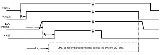
Figure 10. Timing Diagram for the Power-Up Sequence
