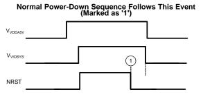
Figure 11. The External Power Control System Deasserts NRST
