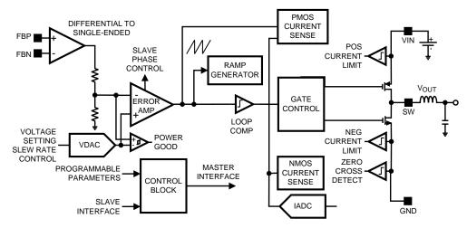
Figure 6. Detailed Block Diagram Showing One Buck Core
