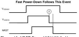
Figure 12. NRST Stays HIGH While V<sub>VIOSYS</sub> Transition from HIGH to LOW Happens (Marked as '2')
