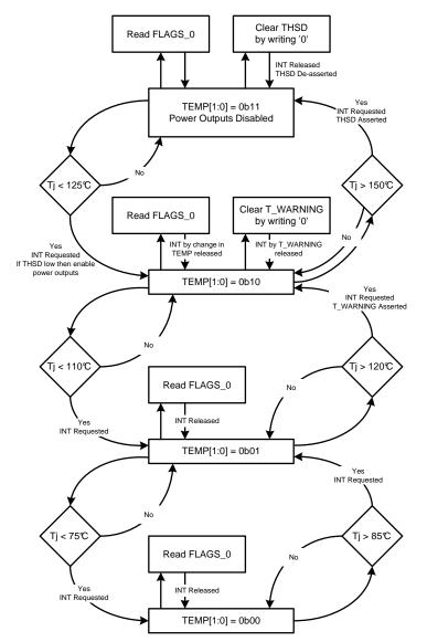
Note that INT is asserted whenever any of the thermal thresholds is crossed, if unmasked. Note also the  $10^{\circ}$ C Hysteresis on the T<sub>J</sub> Thresholds.
