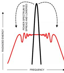
Where a fixed-frequency converter exhibits large amounts of spectral energy at the switching frequency, the spread spectrum architecture of the LP8755 spreads that energy over a large bandwidth.
