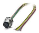
Sensor/actuator flush-type socket, 8-pos., M12 SPEEDCON, rear/screw mounting with M16 thread, with 0.5 m TPE litz wire, 8 x 0.25 mm²
