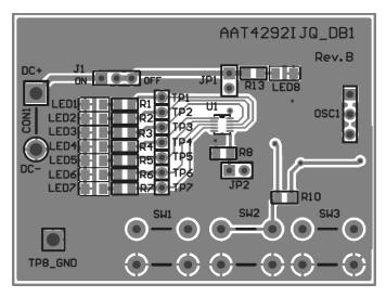
Figure 5: AAT4292 Evaluation Board Layout Top Layer (not to scale).
