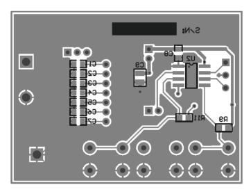
Figure 6: AAT4292 Evaluation Board Layout Bottom Layer (not to scale).
