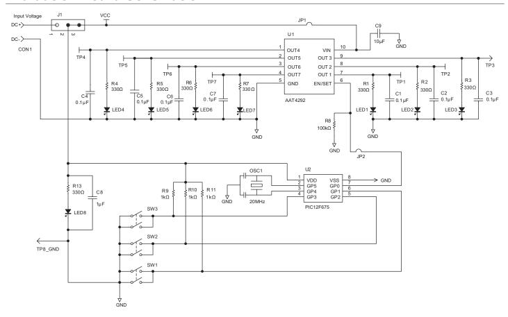
Figure 4: AAT4292 Evaluation Board Schematic.
