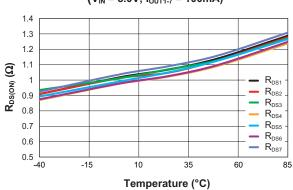
$\begin{array}{l} R_{DS(ON)} \ vs. \ Temperature \\ \left(V_{IN} = 5.0V; \ I_{OUT1-7} = 10mA) \end{array}$
