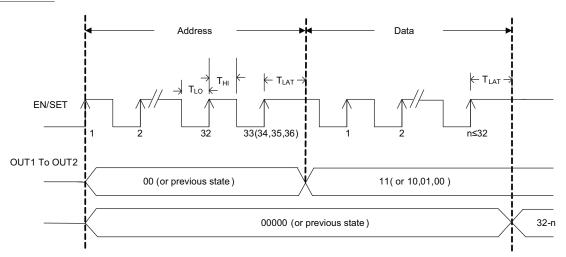
Figure 1: AS<sup>2</sup>Cwire Timing Diagram.
