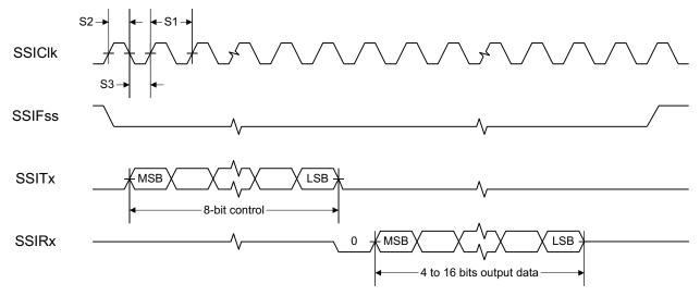
Figure 5-2. SSI Timing for MICROWIRE Frame Format (FRF = 10), Single Transfer
