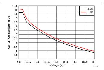
Figure 5-10. TX Current Consumption vs Supply Voltage (VDDS)
