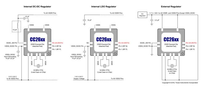
Figure 7-2. Supply Voltage Configurations
