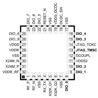
Note: I/O pins marked in bold have high drive capabilities. I/O pins marked in italics have analog capabilities.
