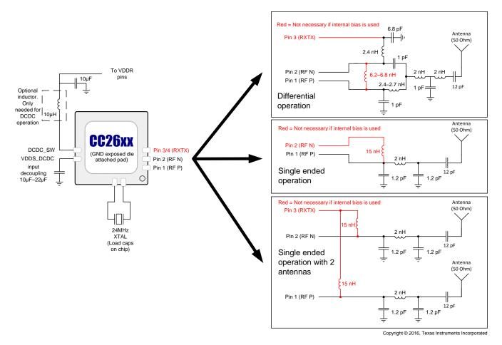
Figure 7-1. CC2620 Application Circuit
