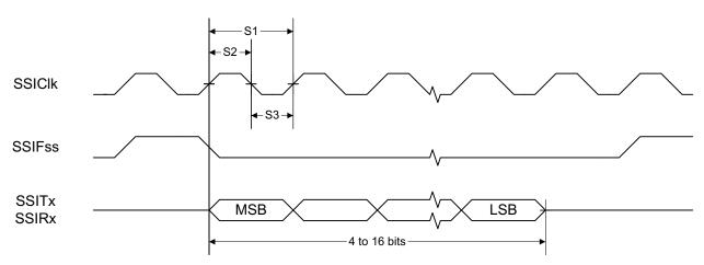
Figure 5-1. SSI Timing for TI Frame Format (FRF = 01), Single Transfer Timing Measurement
