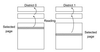
The data transfer operation from the cell array to the Data Cache via Page Buffer starts on the rising edge of WE in the 30h command input cycle (after the 2 Districts' address information has been latched). The device will be in the Busy state during this transfer period.
