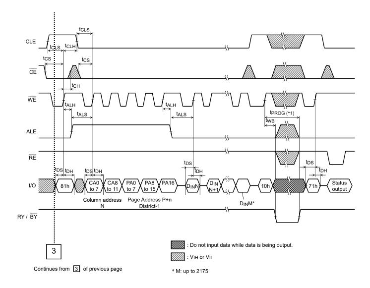
(\*1) tPROG: Since the last page's programming by 10h command is initiated after the previous cache program, the tPROG during cache programming is given by the following equation.
