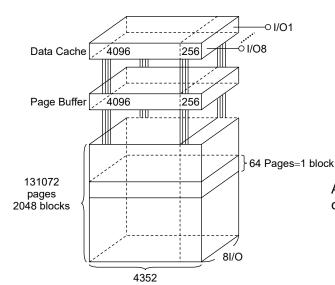
A page consists of 4352 bytes in which 4096 bytes are used for main memory storage and 256 bytes are for redundancy or for other uses.
