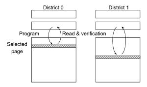
The data is transferred (programmed) from the page buffer to the selected page on the rising edge of /WE following input of the "15h" or "10h" command. After programming, the programmed data is transferred back to the register to be automatically verified by the device. If the programming does not succeed, the Program/Verify operation is repeated by the device until success is achieved or until the maximum loop number set in the device is reached.
