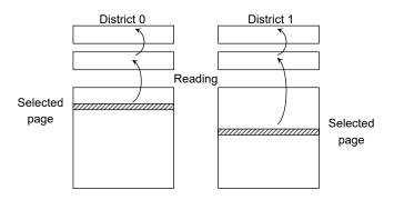
The data transfer operation from the cell array to the Data Cache via Page Buffer starts on the rising edge of WE in the 30h command input cycle (after the 2 Districts' address information has been latched). The device will be in the Busy state during this transfer period.
