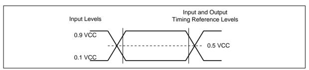
Figure 59. AC Measurement I/O Waveform
