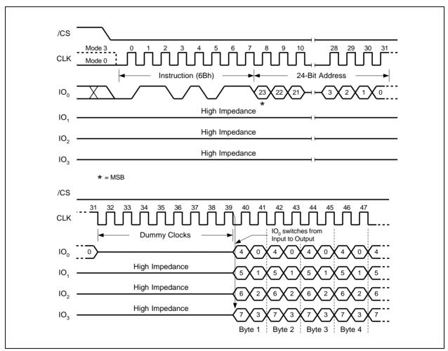
Figure 20. Fast Read Quad Output Instruction
