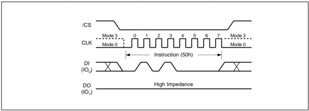
Figure 6. Write Enable for Volatile Status Register Instruction
