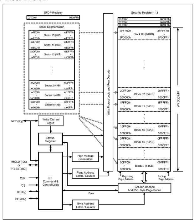
Figure 2. W25Q32JV Serial Flash Memory Block Diagram
