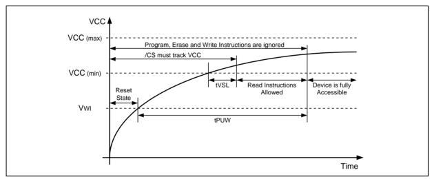
Figure 58a. Power-up Timing and Voltage Levels
