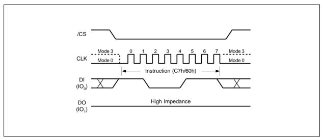
Figure 34. Chip Erase Instruction Sequence Diagram
