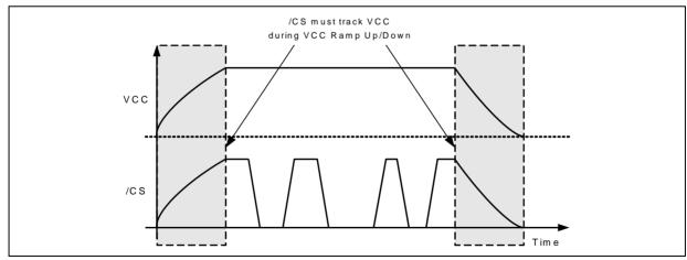
Figure 58b. Power-up, Power-Down Requirement
