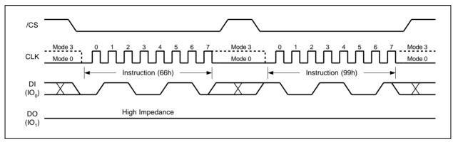
Figure 58. Enable Reset and Reset Instruction Sequence
