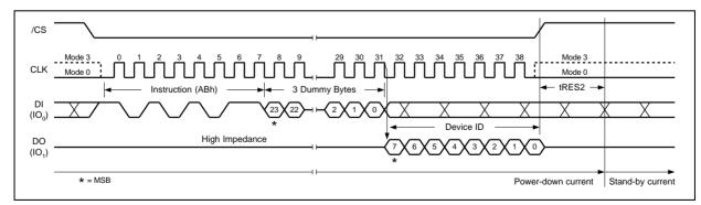
Figure 38b. Release Power-down / Device ID Instruction
