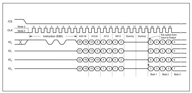
Figure 24. Fast Read Quad I/O Instruction (M7-M0 should be set to Fxh)
