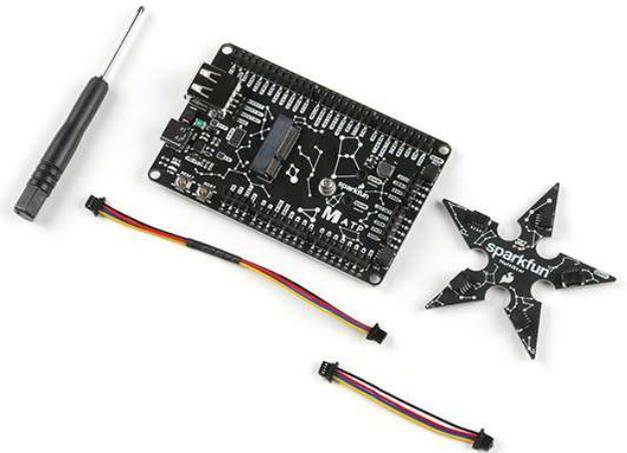
Access all the pins (i.e. ATP) of the MicroMod Processor Boards with the SparkFun MicroMod ATP Carrier Board.
