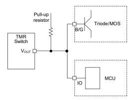
Figure 10. Application diagram for driving power load
