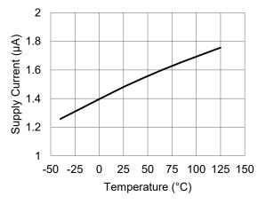
Figure 7. Supply current versus temperature ( $V_{CC}$  = 3 V)
