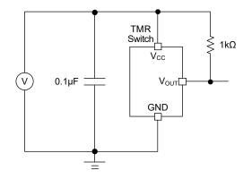
Figure 9. Application circuit diagram
