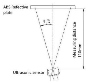
During the test, the launch angle is perpendicular to the plate as a base, then shift the sensor to the left or right for testing.
