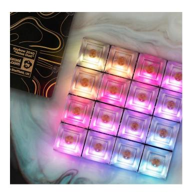
A luxe all-in-one 16 key mini mechanical keyboard with hot swap clicky or linear switches and per key customizable RGB lighting.
