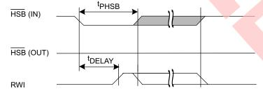
$\overline{\text{HSB}}$  pin is driven  $\underline{\text{HIGH}}$  to  $\overline{\text{V}_{CC}}$  only by Internal 100 KΩ resistor,  $\overline{\text{HSB}}$  driver is disabled SRAM is disabled as long as  $\overline{\text{HSB}}$  (IN) is driven LOW.
