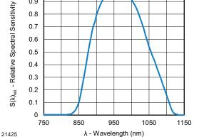
Fig. 7 - Relative Spectral Sensitivity vs. Wavelength
