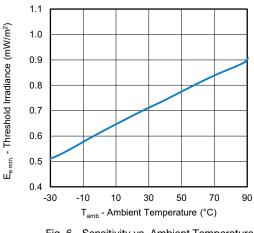
Fig. 6 - Sensitivity vs. Ambient Temperature
