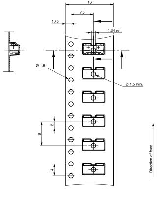
Drawing-No.: 9.700-5337.01-4 Issue: 2; 06.10.15 technical drawings according to DIN specifications
