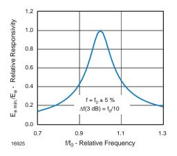
Fig. 5 - Frequency Dependence of Responsivity
