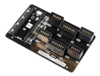
An easy, solderless, swappable way to use breakouts with your Raspberry Pi Pico - add up to six Pimoroni breakouts (4 x I2C and 2 x SPI) to the sturdy slots and get coding and creating!
