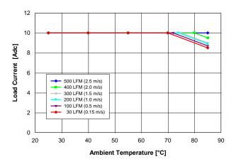
Fig. 5.0V.1: Available load current vs. ambient temperature and airflow rates for Vout = 5.0 V converter mounted vertically with Vin = 12 V, and maximum MOSFET temperature ≤ 110 °C.
