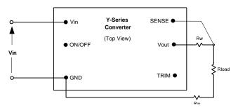
Fig. B: Circuit configuration for ON/OFF function.
