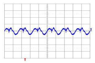
Fig. 1.5V.6: Output voltage ripple (20 mV/div.) at full rated load current into a resistive load with external capacitance  $100 \, \mu F$  ceramic +  $1 \, \mu F$  ceramic, and  $Vin = 12 \, V$  for  $Vout = 1.5 \, V$ . Time scale:  $2 \, \mu s$ /div.
