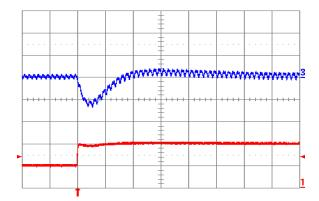
Fig. 2.5V.7: Output voltage response for Vout = 2.5 V to positive load current step change from 5 A to 10 A with slew rate of 5 A/μs at Vin = 12 V. Top trace: output voltage (100 mV/div.); Bottom trace: load current (5 A/div.). Co = 100 μF ceramic. Time scale: 20 μs/div.
