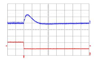
Fig. 2.0V.8: Output voltage response for Vout = 2.0 V to negative load current step change from 10 A to 5 A with slew rate of -5 A/μs at Vin = 12 V. Top trace: output voltage (100 mV/div.); Bottom trace: load current (5 A/div.). Co = 100 μF ceramic. Time scale: 20 μs/div.
