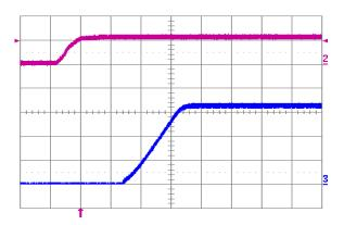
Fig. 3.3V.5: Turn-on transient for Vout = 3.3 V with application of Vin at full rated load current (resistive) and 100 μF external capacitance at Vin = 12 V. Top trace: Vin (10 V/div.); Bottom trace: output voltage (1 V/div.); Time scale: 2 ms/div.
