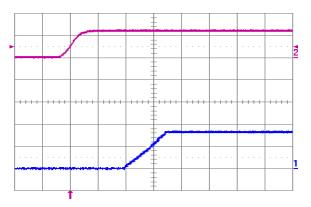
Fig. 0.7525V.5: Turn-on transient for Vout = 0.7525 V with application of Vin at full rated load current (resistive) and 100 μF external capacitance at Vin = 12 V. Top trace: Vin (10 V/div.); Bottom trace: output voltage (0.5 V/div.); Time scale: 2 ms/div.
