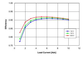
Fig. 1.8V.3: Efficiency vs. load current and input voltage for Vout = 1.8 V converter mounted vertically with air flowing at a rate of 200 LFM (1 m/s) and Ta = 25 °C.
