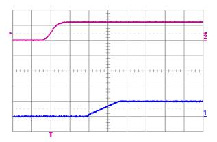
Fig. 1.0V.5: Turn-on transient for Vout = 1.0 V with application of Vin at full rated load current (resistive) and 100 μF external capacitance at Vin = 12 V. Top trace: Vin (10 V/div.); Bottom trace: output voltage (1 V/div.); Time scale: 2 ms/div.
