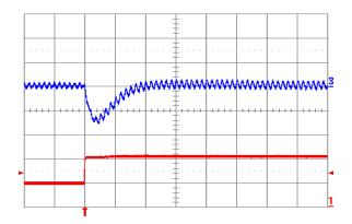
Fig. 5.0V.7: Output voltage response for Vout = 5.0 V to positive load current step change from 5 A to 10 A with slew rate of 5 A/μs at Vin = 12 V. Top trace: output voltage (100 mV/div.); Bottom trace: load current (5 A/div.). Co = 100 μF ceramic. Time scale: 20 μs/div.
