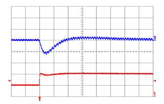
Fig. 1.2V.7: Output voltage response for Vout = 1.2 V to positive load current step change from 5 A to 10 A with slew rate of 5 A/μs at Vin = 12 V. Top trace: output voltage (100 mV/div.); Bottom trace: load current (5 A/div.). Co = 100 μF ceramic. Time scale: 20 μs/div.
