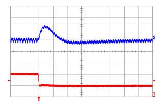
Fig. 2.5V.8: Output voltage response for Vout = 2.5 V to negative load current step change from 10 A to 5 A with slew rate of -5 A/μs at Vin = 12 V. Top trace: output voltage (100 mV/div.); Bottom trace: load current (5 A/div.). Co = 100 μF ceramic. Time scale: 20 μs/div.
