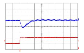
Fig. 2.0V.7: Output voltage response for Vout = 2.0 V to positive load current step change from 5 A to 10 A with slew rate of 5 A/μs at Vin = 12 V. Top trace: output voltage (100 mV/div.); Bottom trace: load current (5 A/div.). Co = 100 μF ceramic. Time scale: 20 μs/div.
