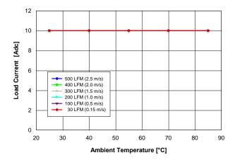
Fig. 0.7525V.2: Available load current vs. ambient temperature and airflow rates for Vout = 0.7525 V converter mounted horizontally with Vin = 12 V, and maximum MOSFET temperature ≤ 110 °C.
