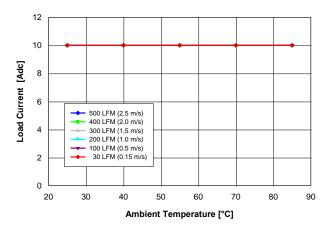
Fig. 2.0V.1: Available load current vs. ambient temperature and airflow rates for Vout = 2.0 V converter mounted vertically with Vin = 12 V, and maximum MOSFET temperature ≤ 110 °C.
