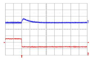
Fig. 1.8V.8: Output voltage response for Vout = 1.8 V to negative load current step change from 10 A to 5 A with slew rate of -5 A/μs at Vin = 12 V. Top trace: output voltage (100 mV/div.); Bottom trace: load current (5 A/div.). Co = 100 μF ceramic. Time scale: 20 μs/div.
