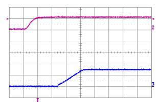
Fig. 1.5V.5: Turn-on transient for Vout = 1.5 V with application of Vin at full rated load current (resistive) and 100 μF external capacitance at Vin = 12 V. Top trace: Vin (10 V/div.); Bottom trace: output voltage (1 V/div.); Time scale: 2 ms/div
