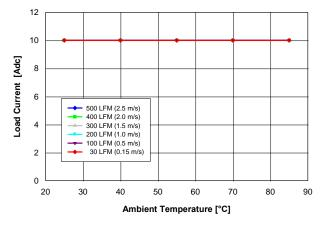
Fig. 0.7525V.1: Available load current vs. ambient temperature and airflow rates for  $Vout = 0.7525 \ V$  converter mounted vertically with  $Vin = 12 \ V$ , and maximum MOSFET temperature  $\leq 110 \ ^{\circ}C$ .
