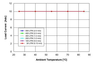
Fig. 2.5V.1: Available load current vs. ambient temperature and airflow rates for Vout = 2.5 V converter mounted vertically with Vin = 12 V, and maximum MOSFET temperature ≤ 110 °C.
