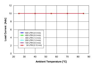
Fig. 1.2V.2: Available load current vs. ambient temperature and airflow rates for Vout = 1.2 V converter mounted horizontally with Vin = 12 V, and maximum MOSFET temperature ≤ 110 °C.
