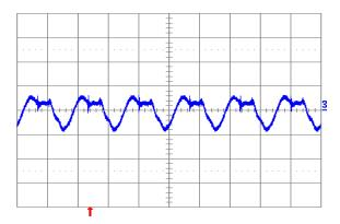
Fig. 2.5V.6: Output voltage ripple (20 mV/div.) at full rated load current into a resistive load with external capacitance 100 μF ceramic + 1 μF ceramic, and Vin = 12 V for Vout = 2.5 V. Time scale: 2 μs/div.
