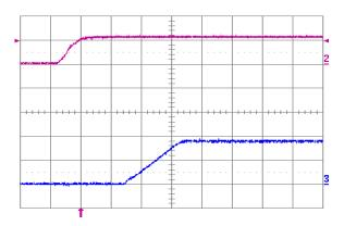
Fig. 1.8V.5: Turn-on transient for Vout = 1.8 V with application of Vin at full rated load current (resistive) and 100 μF external capacitance at Vin = 12 V. Top trace: Vin (10 V/div.); Bottom trace: output voltage (1 V/div.); Time scale: 2 ms/div.
