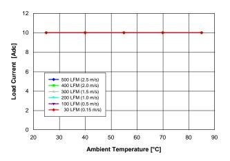
Fig. 2.0V.2: Available load current vs. ambient temperature and airflow rates for Vout = 2.0 V converter mounted horizontally with Vin = 12 V, and maximum MOSFET temperature ≤ 110 °C.
