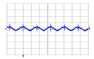
Fig. 1.0V.6: Output voltage ripple (20 mV/div.) at full rated load current into a resistive load with external capacitance  $100 \, \mu F$  ceramic +  $1 \, \mu F$  ceramic, and  $Vin = 12 \, V$  for  $Vout = 1.0 \, V$ . Time scale:  $2 \, \mu s$ /div.
