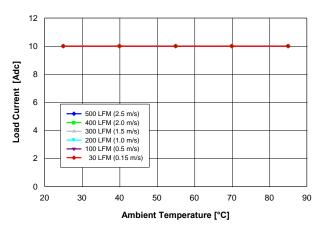
Fig. 1.0V.1: Available load current vs. ambient temperature and airflow rates for Vout = 1.0 V converter mounted vertically with Vin = 12 V, and maximum MOSFET temperature ≤ 110 °C.
