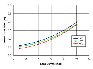
Fig. 2.0V.4: Power Loss vs. load current and input voltage for Vout = 2.0 V converter mounted vertically with air flowing at a rate of 200 LFM (1 m/s) and Ta = 25 °C.
