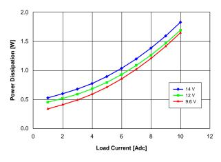
Fig. 1.5V.4: Power Loss vs. load current and input voltage for Vout = 1.5 V converter mounted vertically with air flowing at a rate of 200 LFM (1 m/s) and Ta = 25 °C.
