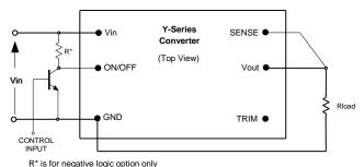
Fig. A: Circuit configuration for ON/OFF function.
