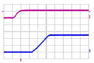
Fig. 2.5V.5: Turn-on transient for Vout = 2.5 V with application of Vin at full rated load current (resistive) and 47 μF external capacitance at Vin = 12 V. Top trace: Vin (10 V/div.); Bottom trace: output voltage (1 V/div.); Time scale: 2 ms/div.
