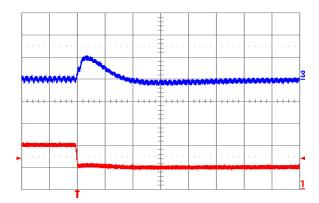
Fig. 1.2V.8: Output voltage response for Vout = 1.2 V to negative load current step change from 10 A to 5 A with slew rate of -5 A/μs at Vin = 12 V. Top trace: output voltage (100 mV/div.); Bottom trace: load current (5 A/div.). Co = 100 μF ceramic. Time scale: 20 μs/div.
