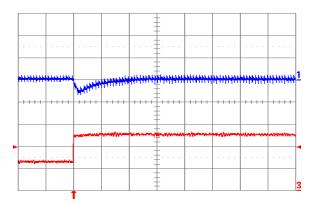
Fig. 1.8V.7: Output voltage response for Vout = 1.8 V to positive load current step change from 5 A to 10 A with slew rate of 5 A/μs at Vin = 12 V. Top trace: output voltage (100 mV/div.); Bottom trace: load current (5 A/div.). Co = 100 μF ceramic. Time scale: 20 μs/div.
