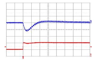
Fig. 1.5V.7: Output voltage response for Vout = 1.5 V to positive load current step change from 5 A to 10 A with slew rate of 5 A/μs at Vin = 12 V. Top trace: output voltage (100 mV/div.); Bottom trace: load current (2 A/div.). Co = 100 μF ceramic. Time scale: 20 μs/div.
