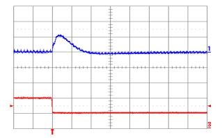
Fig. 0.7525V.8: Output voltage response for Vout = 0.7525 V to negative load current step change from 10 A to 5 A with slew rate of -5 A/μs at Vin = 12 V. Top trace: output voltage (100 mV/div.); Bottom trace: load current (5 A/div.). Co = 100 μF ceramic. Time scale: 20 μs/div.
