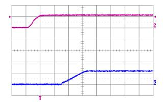
Fig. 1.2V.5: Turn-on transient for Vout = 1.2 V with application of Vin at full rated load current (resistive) and 100 μF external capacitance at Vin = 12 V. Top trace: Vin (10 V/div.); Bottom trace: output voltage (1 V/div.); Time scale: 5 ms/div.
