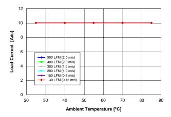
Fig. 2.5V.2: Available load current vs. ambient temperature and airflow rates for Vout = 2.5 V converter mounted horizontally with Vin = 12 V, and maximum MOSFET temperature ≤ 110 °C.
