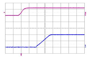
Fig. 2.0V.5: Turn-on transient for Vout = 2.0 V with application of Vin at full rated load current (resistive) and 100 μF external capacitance at Vin = 12 V. Top trace: Vin (10 V/div.); Bottom trace: output voltage (1 V/div.); Time scale: 2 ms/div.
