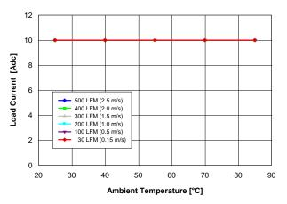
Fig. 3.3V.2: Available load current vs. ambient temperature and airflow rates for Vout = 3.3 V converter mounted horizontally with Vin = 12 V, and maximum MOSFET temperature ≤ 110 °C.
