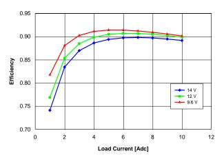
Fig. 1.5V.3: Efficiency vs. load current and input voltage for Vout = 1.5 V converter mounted vertically with air flowing at a rate of 200 LFM (1 m/s) and Ta = 25 °C.
