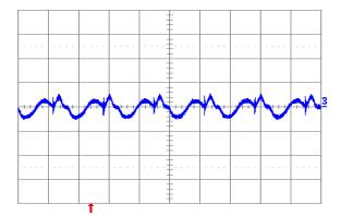
Fig. 1.2V.6: Output voltage ripple (20 mV/div.) at full rated load current into a resistive load with external capacitance  $100 \, \mu F$  ceramic +  $1 \, \mu F$  ceramic, and  $Vin = 12 \, V$  for  $Vout = 1.2 \, V$ . Time scale:  $2 \, \mu s$ /div.
