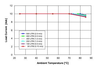
Fig. 5.0V.2: Available load current vs. ambient temperature and airflow rates for Vout = 5.0 V converter mounted horizontally with Vin = 12 V, and maximum MOSFET temperature ≤ 110 °C.
