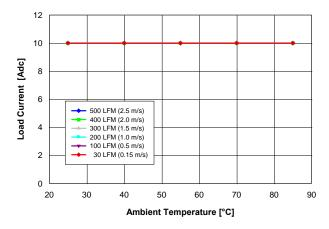
Fig. 1.0V.2: Available load current vs. ambient temperature and airflow rates for Vout = 1.0 V converter mounted horizontally with Vin = 12 V, and maximum MOSFET temperature ≤ 110 °C.
