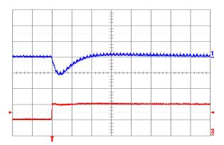
Fig. 1.0V.7: Output voltage response for Vout = 1.0 V to positive load current step change from 5 A to 10 A with slew rate of 5 A/μs at Vin = 12 V. Top trace: output voltage (100 mV/div.); Bottom trace: load current (5 A/div.). Co = 100 μF ceramic. Time scale: 20 μs/div.
