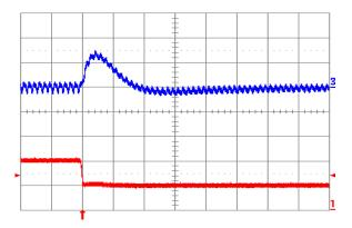
Fig. 3.3V.8: Output voltage response for Vout = 3.3 V to negative load current step change from 10 A to 5 A with slew rate of -5 A/μs at Vin = 12 V. Top trace: output voltage (100 mV/div.); Bottom trace: load current (2 A/div.). Co = 100 μF ceramic. Time scale: 20 μs/div.
