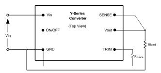
Fig. C: Configuration for programming output voltage.
