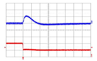
Fig. 1.5V.8: Output voltage response for Vout = 1.5 V to negative load current step change from 10 A to 5 A with slew rate of -5 A/μs at Vin = 12 V. Top trace: output voltage (100 mV/div.); Bottom trace: load current (2 A/div.). Co = 100 μF ceramic. Time scale: 20 μs/div.
