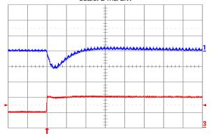
Fig. 0.7525V.7: Output voltage response for Vout = 0.7525 V to positive load current step change from 5 A to 10 A with slew rate of 5 A/μs at Vin = 12 V. Top trace: output voltage (100 mV/div.); Bottom trace: load current (5 A/div.). Co = 100 μF ceramic. Time scale: 20 μs/div.
