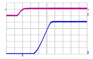
Fig. 5.0V.5: Turn-on transient for Vout = 5.0 V with application of Vin at full rated load current (resistive) and 100 μF external capacitance at Vin = 12 V. Top trace: Vin (10 V/div.); Bottom trace: output voltage (1 V/div.); Time scale: 2 ms/div.
