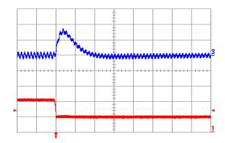
Fig. 5.0V.8: Output voltage response for Vout = 5.0 V to negative load current step change from 10 A to 5 A with slew rate of -5 A/μs at Vin = 12 V. Top trace: output voltage (100 mV/div.); Bottom trace: load current (5 A/div.). Co = 100 μF ceramic. Time scale: 20 μs/div.
