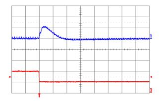
Fig. 1.0V.8: Output voltage response for Vout = 1.0 V to negative load current step change from 10 A to 5 A with slew rate of -5 A/μs at Vin = 12 V. Top trace: output voltage (100 mV/div.); Bottom trace: load current (5 A/div.). Co = 100 μF ceramic. Time scale: 20 μs/div.
