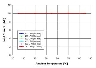
Fig. 3.3V.1: Available load current vs. ambient temperature and airflow rates for Vout = 3.3 V converter mounted vertically with Vin = 12 V, and maximum MOSFET temperature ≤ 110 °C.
