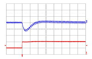
Fig. 3.3V.7: Output voltage response for Vout = 3.3 V to positive load current step change from 5 A to 10 A with slew rate of 5 A/μs at Vin = 12 V. Top trace: output voltage (100 mV/div.); Bottom trace: load current (5 A/div.). Co = 100 μF ceramic. Time scale: 20 μs/div.
