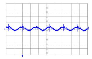
Fig. 0.7525V.6: Output voltage ripple (20 mV/div.) at full rated load current into a resistive load with external capacitance  $100 \,\mu\text{F}$  ceramic +  $1 \,\mu\text{F}$  ceramic, and Vin =  $12 \,\text{V}$  for Vout =  $0.7525 \,\text{V}$ . Time scale:  $2 \,\mu\text{s}/\text{div}$ .
