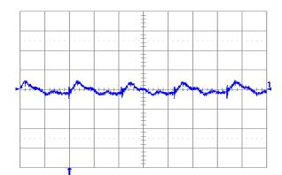
Fig. 1.8V.6: Output voltage ripple (20 mV/div.) at full rated load current into a resistive load with external capacitance 47μF ceramic + 1μF ceramic, and Vin = 12 V for Vout = 1.8 V. Time scale: 1 μs/div.
