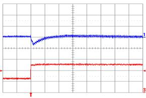
Fig. 2.5V.7: Output voltage response for Vout = 2.5 V to positive load current step change from 2.5 A to 5 A with slew rate of 5 A/μs at Vin = 12 V. Top trace: output voltage (100 mV/div.); Bottom trace: load current (2 A/div.). Co = 47 μF ceramic. Time scale: 20 μs/div.
