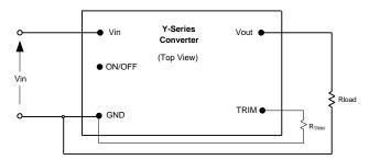
Fig. B. Configuration for programming output voltage.
