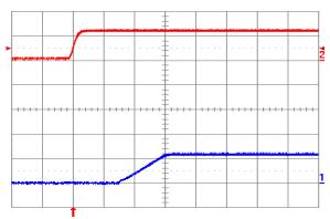
Fig. 1.2V.5: Turn-on transient for Vout = 1.2 V with application of Vin at full rated load current (resistive) and 47 μF external capacitance at Vin = 12 V. Top trace: Vin (10 V/div.); Bottom trace: output voltage (1 V/div.); Time scale: 5 ms/div.
