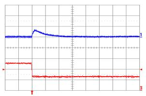
Fig. 1.5V.8: Output voltage response for Vout = 1.5 V to negative load current step change from 5 A to 2.5 A with slew rate of -5 A/ $\mu$ s at Vin = 12 V. Top trace: output voltage (100 mV/div.); Bottom trace: load current (2 A/div.). Co = 47  $\mu$ F ceramic. Time scale: 20  $\mu$ s/div.
