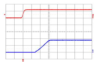
Fig. 1.8V.5: Turn-on transient for Vout = 1.8 V with application of Vin at full rated load current (resistive) and 47 μF external capacitance at Vin = 12 V. Top trace: Vin (10 V/div.); Bottom trace: output voltage (1 V/div.); Time scale: 5 ms/div.
