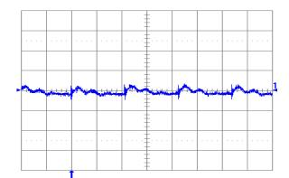
Fig. 1.0V.6: Output voltage ripple (20 mV/div.) at full rated load current into a resistive load with external capacitance 47 μF ceramic + 1 μF ceramic, and Vin = 12 V for Vout = 1.0 V. Time scale: 1 μs/div.
