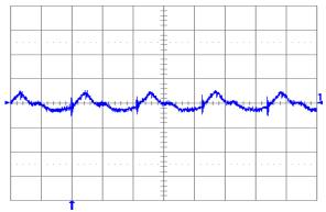
Fig. 2.5V.6: Output voltage ripple (20 mV/div.) at full rated load current into a resistive load with external capacitance 47 μF ceramic + 1 μF ceramic, and Vin = 12 V for Vout = 2.5 V. Time scale: 1 μs/div.
