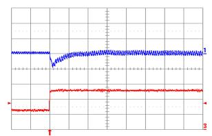
Fig. 5.0V.7: Output voltage response for Vout = 5.0 V to positive load current step change from 2.5 A to 5 A with slew rate of 5 A/μs at Vin = 12 V. Top trace: output voltage (100 mV/div.); Bottom trace: load current (2 A/div.). Co = 47 μF ceramic. Time scale: 20 μs/div.
