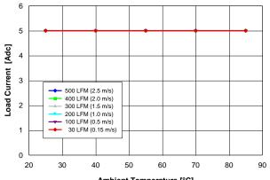
Ambient Temperature [°C] Fig. 1.0V.1: Available load current vs. ambient temperature
