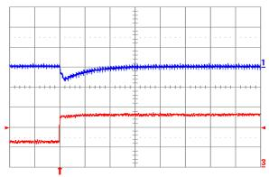
Fig. 1.0V.7: Output voltage response for Vout = 1.0 V to positive load current step change from 2.5 A to 5 A with slew rate of 5 A/μs at Vin = 12 V. Top trace: output voltage (100 mV/div.); Bottom trace: load current (2 A/div.). Co =47 μF ceramic. Time scale: 20 μs/div.
