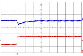
Fig. 1.5V.7: Output voltage response for Vout = 1.5 V to positive load current step change from 2.5 A to 5 A with slew rate of 5 A/μs at Vin = 12 V. Top trace: output voltage (100 mV/div.); Bottom trace: load current (2 A/div.). Co = 47 μF ceramic. Time scale: 20 μs/div.
