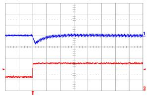
Fig. 3.3V.7: Output voltage response for Vout = 3.3 V to positive load current step change from 2.5 A to 5 A with slew rate of 5 A/μs at Vin = 12 V. Top trace: output voltage (100 mV/div.); Bottom trace: load current (2 A/div.). Co = 47 μF ceramic. Time scale: 20 μs/div.
