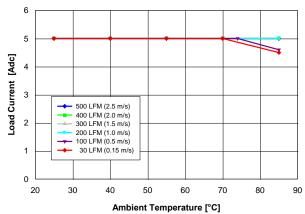
Fig. 5.0V.2: Available load current vs. ambient temperature and airflow rates for Vout = 5.0 V converter mounted horizontally with Vin = 12 V, and maximum MOSFET temperature ≤ 120 °C.
