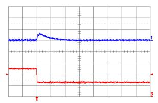
Fig. 2.0V.8: Output voltage response for Vout = 2.0 V to negative load current step change from 5 A to 2.5 A with slew rate of -5 A/ $\mu$ s at Vin = 12 V. Top trace: output voltage (100 mV/div.); Bottom trace: load current (2 A/div.). Co = 47  $\mu$ F ceramic. Time scale: 20  $\mu$ s/div.
