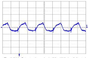
Fig. 5.0V.6: Output voltage ripple (20 mV/div.) at full rated load current into a resistive load with external capacitance  $47 \,\mu F$  ceramic + 1  $\mu F$  ceramic, and Vin = 12 V for Vout = 5.0 V. Time scale: 1  $\mu$ s/div.
