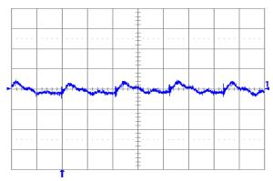
Fig. 1.5V.6: Output voltage ripple (20 mV/div.) at full rated load current into a resistive load with external capacitance 47 μF ceramic + 1 μF ceramic, and Vin = 12 V for Vout = 1.5 V. Time scale: 1 μs/div.
