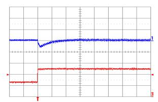
Fig. 2.0V.7: Output voltage response for Vout = 2.0 V to positive load current step change from 2.5 A to 5 A with slew rate of 5 A/μs at Vin = 12 V. Top trace: output voltage (100 mV/div.); Bottom trace: load current (2 A/div.). Co = 47 μF ceramic. Time scale: 20 μs/div.
