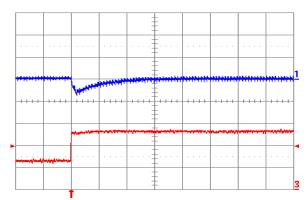
Fig. 1.2V.7: Output voltage response for Vout = 1.2 V to positive load current step change from 2.5 A to 5 A with slew rate of 5 A/μs at Vin = 12 V. Top trace: output voltage (100 mV/div.); Bottom trace: load current (2 A/div.). Co = 47 μF ceramic. Time scale: 20 μs/div.
