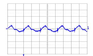
Fig. 3.3V.6: Output voltage ripple (20 mV/div.) at full rated load current into a resistive load with external capacitance 47 μF ceramic + 1 μF ceramic, and Vin = 12 V for Vout = 3.3 V. Time scale: 1 μs/div.
