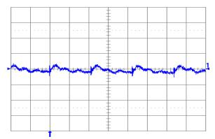
Fig. 1.2V.6: Output voltage ripple (20 mV/div.) at full rated load current into a resistive load with external capacitance 47 μF ceramic + 1 μF ceramic, and Vin = 12 V for Vout = 1.2 V. Time scale: 1 μs/div.
