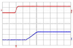
Fig. 1.5V.5: Turn-on transient for Vout = 1.5 V with application of Vin at full rated load current (resistive) and 47 μF external capacitance at Vin = 12 V. Top trace: Vin (10 V/div.); Bottom trace: output voltage (1 V/div.); Time scale: 5 ms/div.
