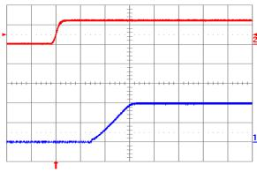
Fig. 2.0V.5: Turn-on transient for Vout = 2.0 V with application of Vin at full rated load current (resistive) and 47 μF external capacitance at Vin = 12 V. Top trace: Vin (10 V/div.); Bottom trace: output voltage (1 V/div.); Time scale: 5 ms/div.
