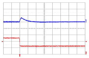
Fig. 2.5V.8: Output voltage response for Vout = 2.5 V to negative load current step change from 5 A to 2.5 A with slew rate of -5 A/ $\mu$ s at Vin = 12 V. Top trace: output voltage (100 mV/div.); Bottom trace: load current (2 A/div.). Co = 47  $\mu$ F ceramic. Time scale: 20  $\mu$ s/div.
