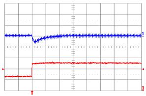
Fig. 1.8V.7: Output voltage response for Vout = 1.8 V to positive load current step change from 2.5 A to 5 A with slew rate of 5 A/μs at Vin = 12 V. Top trace: output voltage (100 mV/div.); Bottom trace: load current (2 A/div.). Co = 47 μF ceramic. Time scale: 20 μs/div.
