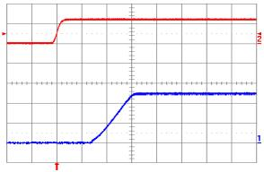
Fig. 2.5V.5: Turn-on transient for Vout = 2.5 V with application of Vin at full rated load current (resistive) and 47 μF external capacitance at Vin = 12 V. Top trace: Vin (10 V/div.); Bottom trace: output voltage (1 V/div.); Time scale: 5 ms/div.
