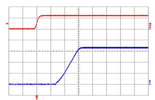
Fig. 3.3V.5: Turn-on transient for Vout = 3.3 V with application of Vin at full rated load current (resistive) and 47 μF external capacitance at Vin = 12 V. Top trace: Vin (10 V/div.); Bottom trace: output voltage (1 V/div.); Time scale: 5 ms/div.
