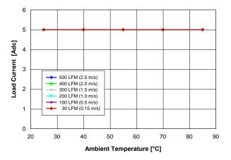
Fig. 2.5V.2: Available load current vs. ambient temperature and airflow rates for Vout = 2.5 V converter mounted horizontally with Vin = 12 V, and maximum MOSFET temperature ≤ 120 °C.
