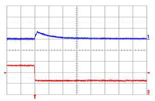
Fig. 1.0V.8: Output voltage response for Vout = 1.0 V to negative load current step change from 5 A to 2.5 A with slew rate of -5 A/ $\mu$ s at Vin = 12 V. Top trace: output voltage (100 mV/div.); Bottom trace: load current (2 A/div.). Co = 47  $\mu$ F ceramic. Time scale: 20  $\mu$ s/div.
