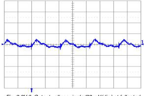
Fig. 2.0V.6: Output voltage ripple (20 mV/div.) at full rated load current into a resistive load with external capacitance  $47 \,\mu F$  ceramic + 1  $\mu F$  ceramic, and Vin = 12 V for Vout = 2.0 V. Time scale: 1  $\mu$ s/div.
