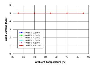
Fig. 2.0V.2: Available load current vs. ambient temperature and airflow rates for Vout = 2.0 V converter mounted horizontally with Vin = 12 V, and maximum MOSFET temperature ≤ 120 °C.
