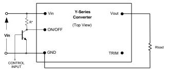
Fig. A. Circuit configuration for ON/OFF function.
