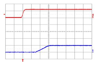
Fig. 1.0V.5: Turn-on transient for Vout = 1.0 V with application of Vin at full rated load current (resistive) and 47 μF external capacitance at Vin = 12 V. Top trace: Vin (10 V/div.); Bottom trace: output voltage (1 V/div.); Time scale: 5 ms/div.
