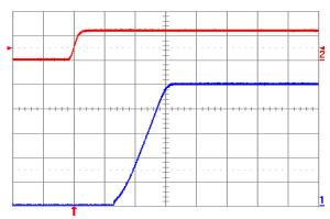
Fig. 5.0V.5: Turn-on transient for Vout = 5.0 V with application of Vin at full rated load current (resistive) and 47 μF external capacitance at Vin = 12 V. Top trace: Vin (10 V/div.); Bottom trace: output voltage (1 V/div.); Time scale: 5 ms/div.
