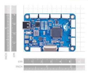
The Ochin CM4 is a tiny carrier board for the Raspberry Pi Compute Module equipped with the powerful Quad-core Cortex-A72 CPU and GPU, which features a big RAM size, the CODECs, and Graphic Accelerators. It's designed for a wide range of applications such as robotics, home automation, and IoT projects.
