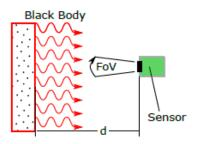
A fluid heated plane black body with an outer dimension covering at least 4 times the sensors field-of-view (FoV) and an emissivity of better than 95% has a surface temperature  $T_{obj}$ . The surface temperature uniformity is better than 0.2 °C. The ambient temperature  $T_{amb}$  is at 25 °C ± 3 °C. The TPIS 1T 1086 L5.5 sensor is mounted at a distance d to the black body. Numbers are specified in table 8.
