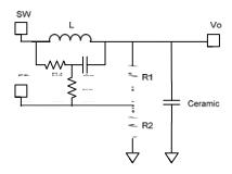
**Figure 8: External Ramp Compensation**
