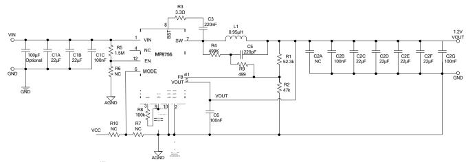
Figure 16: VIN = 12V<sup>(6)</sup>, Vo = 1.2V, Io = 6A Application Schematic with Ceramic Output Capacitors
