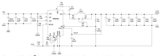
Figure 12: VIN = 12V<sup>(6)</sup>, Vo = 3.3V, Io = 6A Application Schematic with Ceramic Output Capacitors
