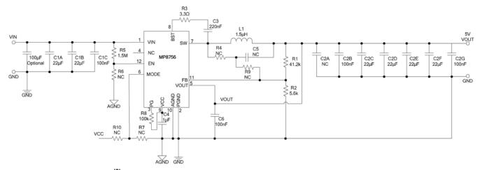
Figure 11: VIN = 12V<sup>(6)</sup>, Vo = 5V, Io = 6A Application Schematic with Ceramic Output Capacitors
