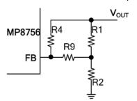
Figure 9: Equivalent DC Circuit
