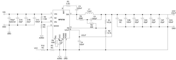
Figure 13: VIN = 12V<sup>6)</sup>, Vo = 2.5V, Io = 6A Application Schematic with Ceramic Output Capacitors
