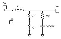
Figure 6: Simplified Circuit of POS Capacitor
