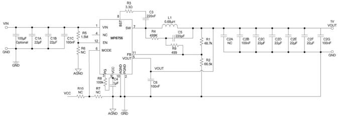
Figure 17: VIN = 12V<sup>(6)</sup>, Vo = 1.0V, Io = 6A Application Schematic with Ceramic Output Capacitors
