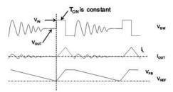
Figure 3: Light-Load Operation
