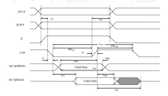
80XX-Series MPU Parallel Interface Timing Characteristics:
