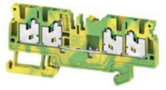
A protective feed through terminal block is an electrical conductor for the purpose of safety and is used in many applications. To establish the electrical and mechanical connection between copper conductors and the mounting support plate, PE terminal blocks are used. They have one or more contact points for connection with and/or bifurcation of protective earth conductors.
