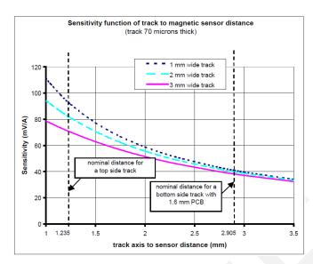
Figure X Sensitivity versus track width and versus distance between the track and the FHS AH sensing elements (TBC)
