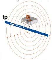
Figure X FHS AH orientation to measure the magnetic field generated by a current along a conductor
