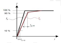
Figure  $\times$  t<sub>D 10</sub> (delay time @ 10 %) and t<sub>D 90</sub> (delay time @ 90 %).
