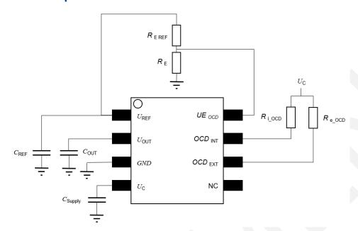
Figure 2 Application circuit
