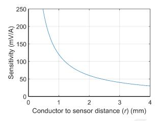
Figure X Sensitivity versus the distance between the conductor and the FHS AH sensing elements
