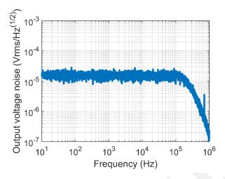
Figure X Output voltage noise
