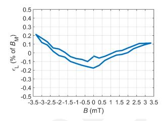
Figure X Linearity error @35 °C
