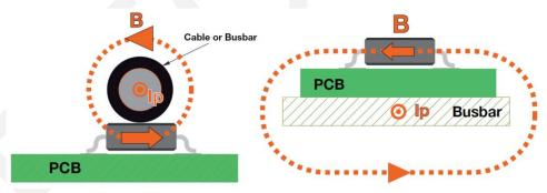
Figure X Example with cable or busbar
