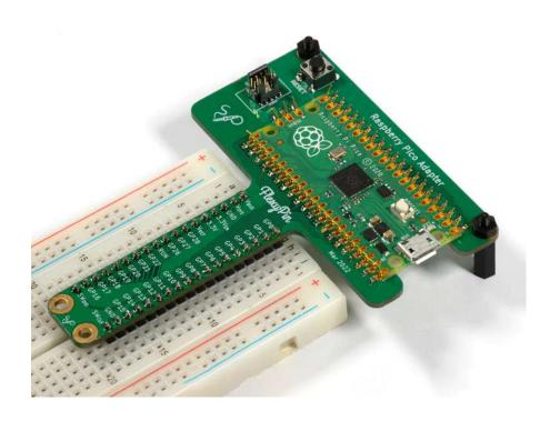
This board allows you to use various modules with a breadboard (and more) without having to solder the module in place. Just add FlexyPins
