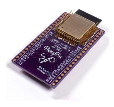
This board allows you to use various modules with a breadboard (and more) without having to solder the module in place. Just add FlexyPins.
