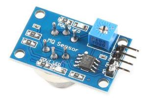
This is the MQ-2 Gas and Smoke Analog Sensor Breakout Board. It's most common use is domestic gas leakage alarms and detectors with a high sensitivity to propane and smoke. The sensing material is  $SNO_2$  (tin oxide) for which the conductivity is lower in clean environments and higher when smoke or flammable gas is present. This is a lowcost sensor for use in a variety of applications.
