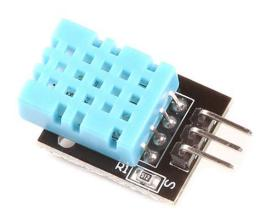
The DHT11 Digital Temperature And Relative Humidity Sensor Module is a low cost humidity and temperature sensor. It can be applied to HVAC, dehumidifier, automatic control, data loggers, weather stations, and many other projects. The sensor is calibrated and doesn't require extra components so you can get right to measuring relative humidity and temperature.
