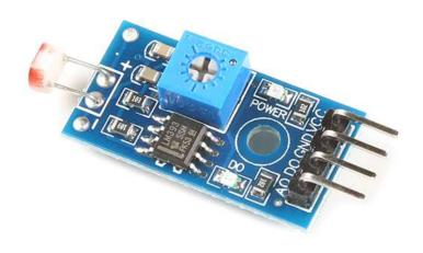
This is a photosensitive resistance module sensitive to ambient light, commonly used for detecting the immediate environment for the brightness of the light, or MCU trigger or relay, etc. Output port can be directly connected to the single-chip microcomputer, through the single-chip microcomputer for detecting level up and down, so the change in intensity of the light of the test environment. End of output can directly drive the relay module, which can form a light switch — operated.
