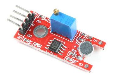
This is a 4-pin microphone voice sound sensor module based around the LM393 chip. It features an electric condenser microphone, single channel signal output with a low level output signal used for sound control light.
